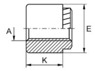
Female thread A = M2,5 Height K = 8 Hole diameter +0.1 = 4.2 Min distance to edge = 2.4 Min material thickness = 1.5 Outer diameter E = 6
